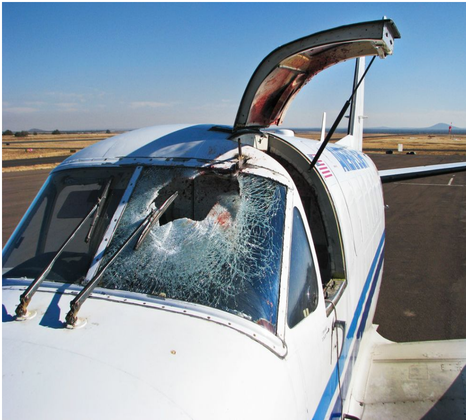
A windshield of a twin-engine Beechcraft C-99 turboprop was splattered with blood after striking a western grebe over Arizona in 2009.
